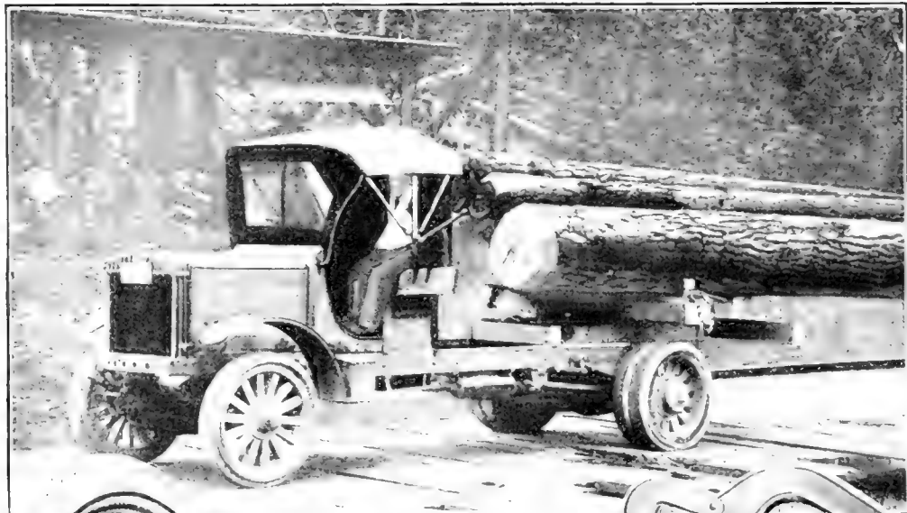
Above: Twelve-ton trees are carried on truck and trailer in Washington. One truck can move about forty-two thousand feet of lumber a day
